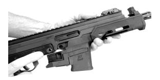
(5) Align retaining pin hole of lower receiver, upper receiver, and Magazine Module and install retaining pin.
