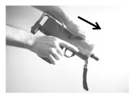
(3) Remove retaining pin and detach upper receiver from lower receiver.
