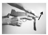
(4) Make sure selector is set to "SMG". This drops the trip down and makes it easier to install the upper. Install upper by aligning the rear of the upper receiver with the rear of the lower receiver, keeping both receivers parallel. Slide on the Magazine Module (G17 Magazine Module shown for reference).
