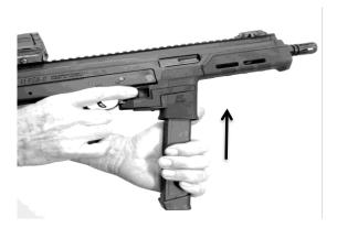
Due to variations in magazines, some magazines may be a snug fit but most will fit loosely. The magazine may have a lot of play after installation, but this will not affect functioning of the VERSA-10.
