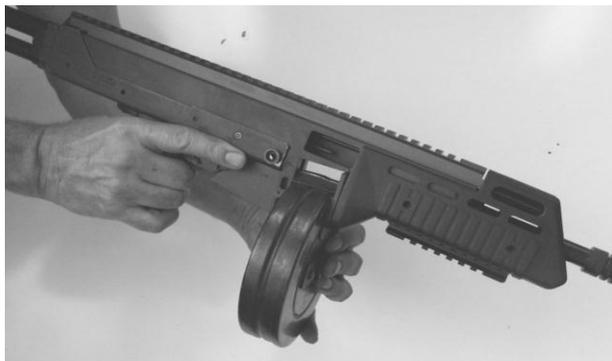
Due to variations in magazines, some magazines may be a snug fit but most will fit loosely. The magazine may have a lot of play after installation, but this will not affect functioning of the MAX-31A.
