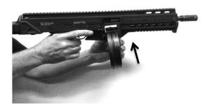
Due to vartiations in magazines, some magazines may be a snug fit but most will fit loosely. The magazine may have a lot of play after installation, but this will not affect functioning of the MAX-31 mk2.
