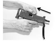
(2) While holding cocking knob, pull trigger and ease bolt forward into closed position.
