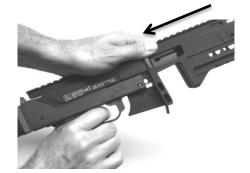
(5) Align retaining pin hole and install retaining pin.
