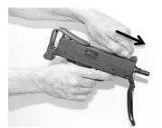
③ Remove retaining pin and detach upper receiver from lower receiver.
