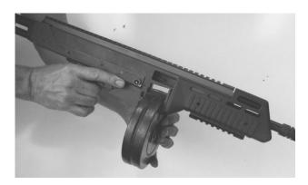
Due to vartiations in magazines, some magazines may be a snug fit but most will fit loosely. The magazine may have a lot of play after installation, but this will not affect functioning of the MAX-31A.
