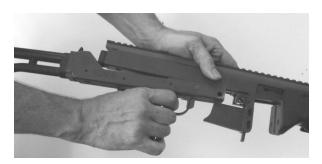
(6) Align retaining pin hole and install retaining pin.
